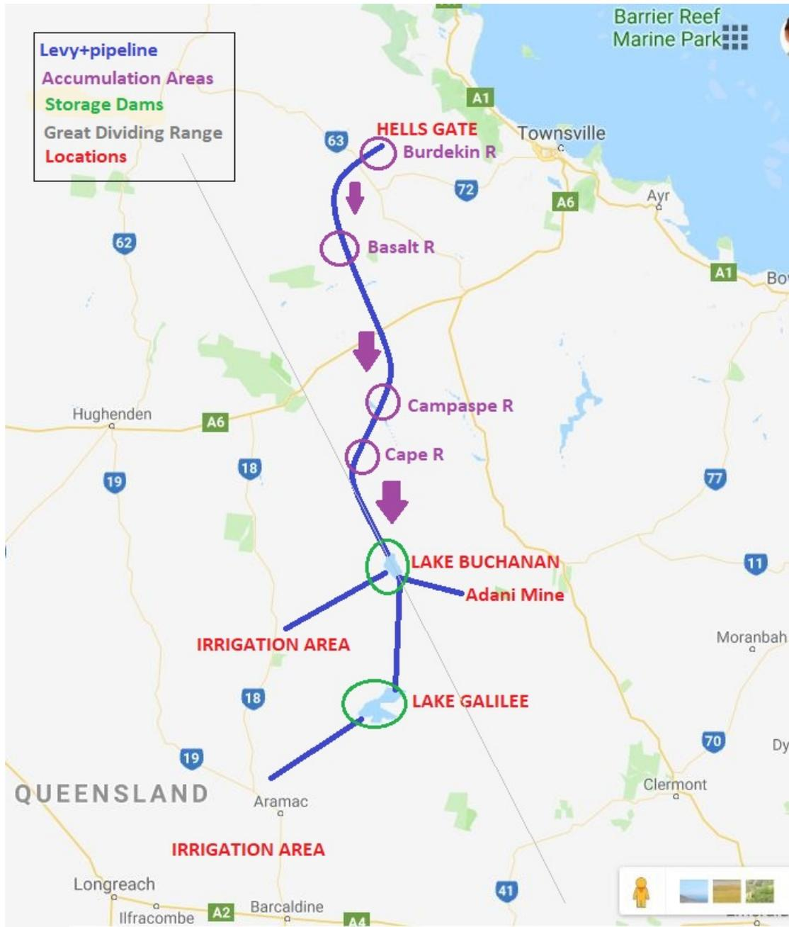
*Illustration 2: Schematic diagram of a gravity-fed mini-Bradfield Scheme transporting water from the coastal rivers via a levy/pipeline combination (blue) to the storage and distribution lakes on the Great Dividing Range (green).*
