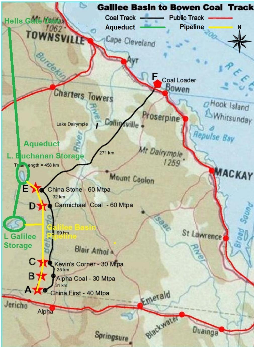
Illustration 3: A Galilee pipeline could be constructed to pipe water from storages and so mitigate the environmental impact of these mines on ground and surface waters.
